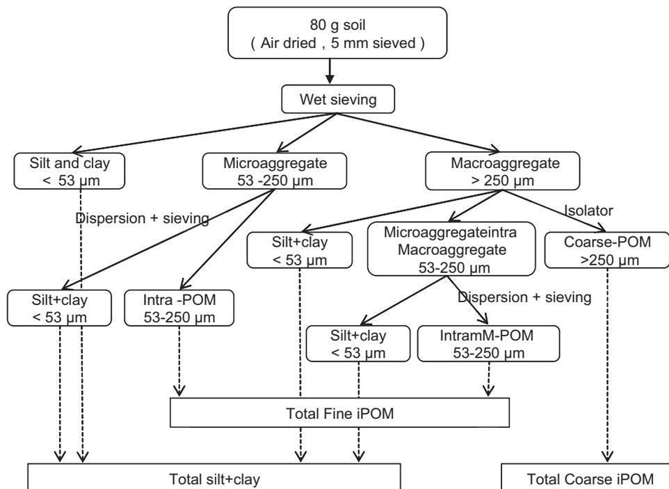
**Fig. 2.** A fractionation scheme to isolate coarse (>250  $\mu\text{m}$ ) intra-aggregate particulate organic matter (iPOM), fine (53–250  $\mu\text{m}$ ) iPOM and (<53  $\mu\text{m}$ ) organomineral complexes (silt + clay).
