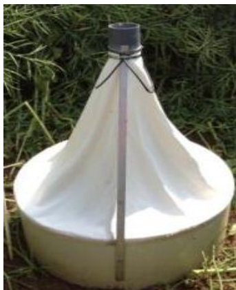
Figure 1. Ground photoelector. The base ring (0.25 m 2 ) is dug into the soil just after winter without disturbing the crop plants within and outside the ring and the tent is fitted at about BBCH 75-78, leaving all plant material grown inside the ring by bending it down before fitting the tent. The electors were then left until harvest date. At the top a trapping box or, for live insect catch, a perforated plastic bag, is fixed to catch all insects escaping through the opening supplying light. For pests such as Dasyneura brassicae and C. napi such traps would have to be established in the crops following oilseed rape.
