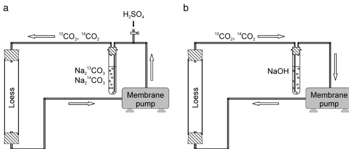
**Fig. 1.** Experimental setup. (a) Labeling procedure:  $^{13}\text{C}$  and  $^{14}\text{C}$  labeled  $\text{CO}_2$  is released by addition of  $\text{H}_3\text{PO}_4$  to the label solution and pumped through the loess sample. (b) Trapping of gaseous  $\text{CO}_2$  in  $\text{NaOH}$  before sampling of the loess.
