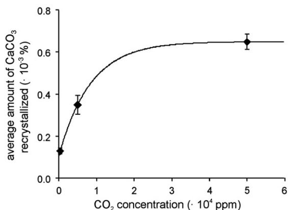
**Fig. 3.** Amount of recrystallized calcium carbonate as percentage of total loess carbonate (averaged from all three sampling dates) depending on  $\text{CO}_2$  concentration.
