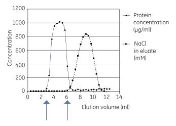
Fig 2. Removal of NaCl from albumin solution with a PD-10 Desalting column. The albumin is eluted in volume fractions between 2.5 and 6.0 ml (indicated by arrows).
