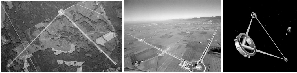
Figure 2.3: Pictures of actual interferometers. The left one is the LIGO interferometer in Livingston (LA, USA) with 4-km-arms. The interferometer in the middle is the Virgo instrument near Pisa (Italy) that has 3-km-arms. The picture on the right is a sketch of the planned LISA interferometer consisting of three satellites at distances of 5 million kilometres [25].
