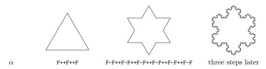
Figure 1: The first steps of the snowflake L-system.
